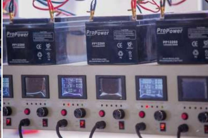
Lead Acid battery testing & recharging system
